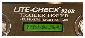
If there is an active fault, the tester will illuminate the ABS lamp on the trailer (CAB ON) and retrieve the fault information.
