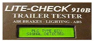
If the trailer ABS controller communicates via the 7-way connector using *power line communications*, (PLC4TRUCKS or PLC), the 910B *INSPECTOR* will detect the signal and automatically communicate with the ABS controller to collect its current status information.
