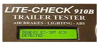
The 910B supports Bendix, Haldex, Wabco and Wabash. The tester will then search the ECU for any faults.
