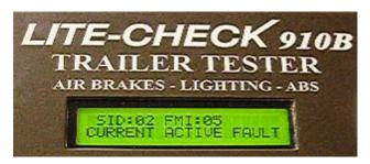
The screen displays the SID & FMI or fault code...
