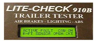
The tester will display the fault (location and description). After this screen appears, pressing the "SELECT" or "D" key on the tester panel will provide additional fault information, and the ABS manufacturer's suggested maintenance steps.
