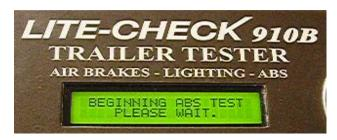
Press the ABS key on the LITE-CHECK 910B //NSPECTOR's control panel to begin the ABS test sequence.
