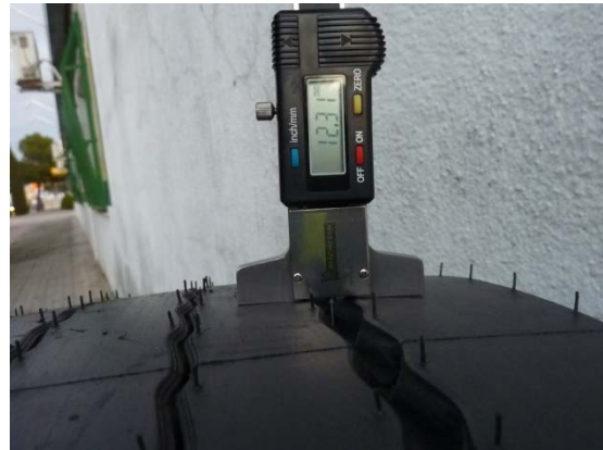
Measuring tread depth in the fully open shoulder grooves on this new tire confirms the same depth of 12.31 mm or 15/32 inch.
